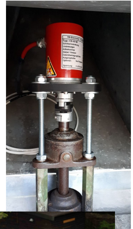
Encoder at secondary spindle spun-off from Az axis
