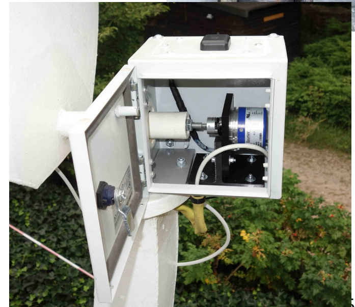
Encoder w/ direct coupling to El axis
