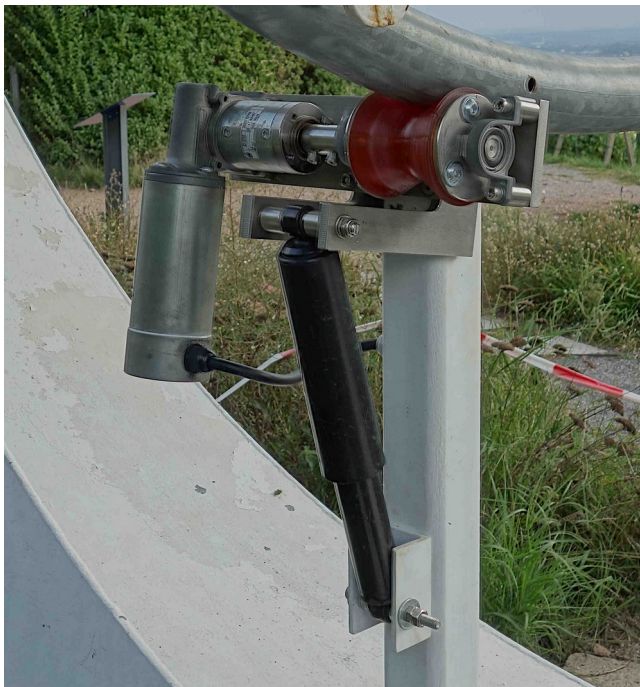
drive of Alt axis – friction clutch
